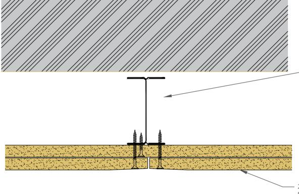
· SPEEDLINE 70mm 'I' Studs at 600mm Ctrs
